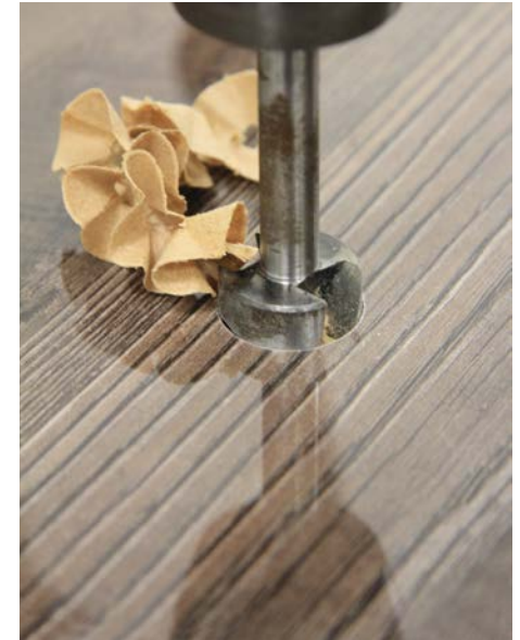
No white fracture/mouse tooth effect
