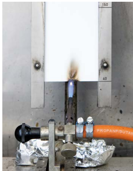
Fire protection testing
